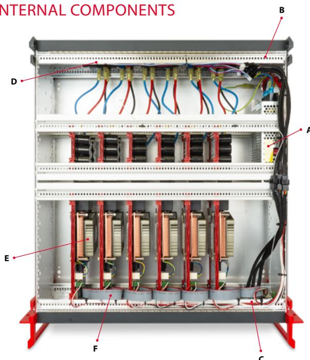
Type C enclosures can host different types of modules, which are commercialized as independent products. One is here shown with 6x PEB8038 half-bridge modules (not included).
