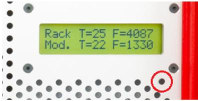
Figure 8. Fault clearing button located under the LCD screen
