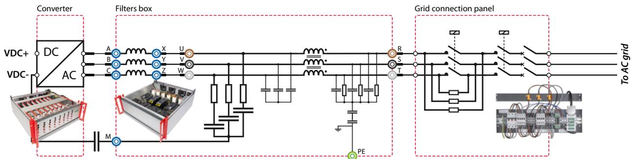
Figure 11. Filter topology for a transformer-less connection to the grid.
