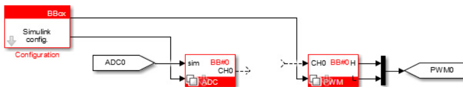
Fig. 20. Connection of the ADC and PWM clocks necessary to provide timing in simulation mode.
